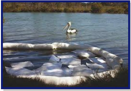
Once the product turns dark brown or black (depending on the oil color), the oil has been captured and can now be recovered using various collection methods and recycled by simply applying pressure and/or compression to the sorbent.
